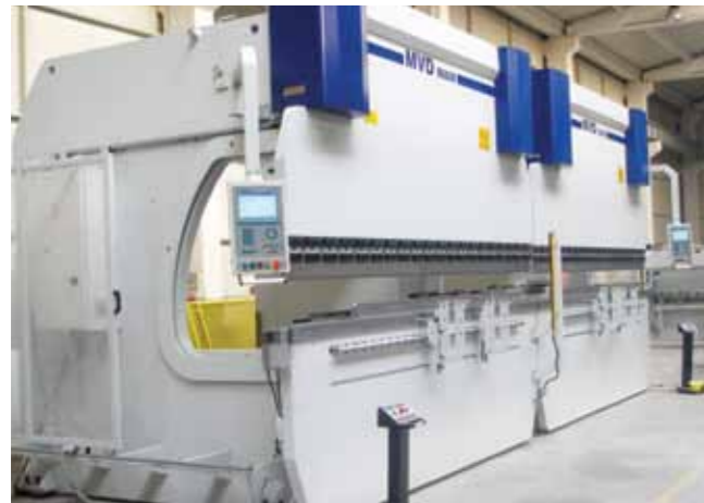
▶ Tandem Machine with 1250mm Throat
